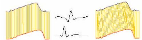
Figure 3. One to one alignment on time axis vs. non-linear alignment (warped time axis). Nonlinear curve alignment is important in pattern recognition of ECG signals. Wavelet analysis dose not allow this type of flexibility in pattern recognition and matching.
